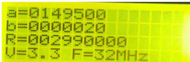
Fig.7. Multiplication result for 8-bit data by LCD.
